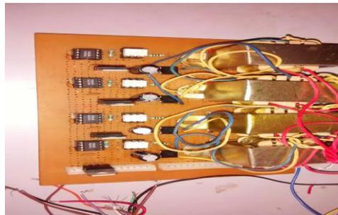
Fig8. Isolation and Driver Circuit.
